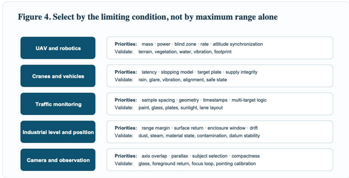
Figure 4. A shorter-range module with better footprint, power, or interface fit may outperform a long-range module in the finished product.
